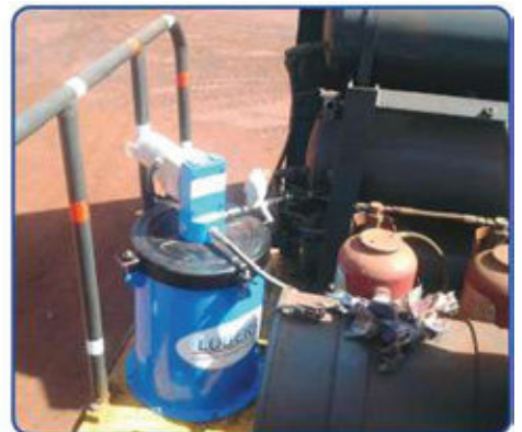
MOTOLUBERR DC operated pump mounted on Top of the Dumper
