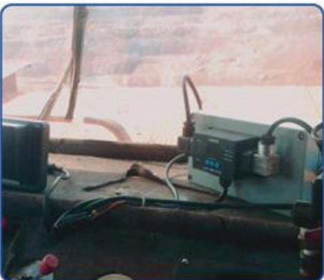
MOTOLUBERR Timer fitted on the Dumper Dash Board for monitoring ALS
