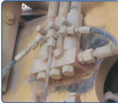
Grease Injector SVM 01 fitted on the Dumper
