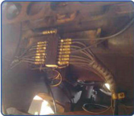
Mono Block Progressive Distributor fitted at the bottom of the Dumper
